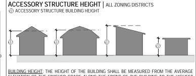
ELEVATION OF THE FINISHED GRADE ALONG THE FRONT OF THE BUILDING TO THE HIGHEST POINT OF THE ROOF OR PARAPET OF THE BUILDING IF IT IS FLAT, MANSARD OR SHED ROOF; OR TO THE MIDPOINT OF THE ROOF IF IT IS GABLE, HIP OR GAMBREL.
